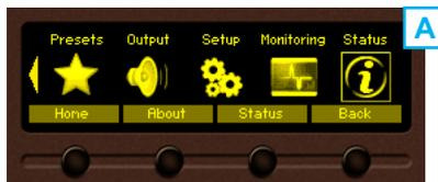
Using the [RIGHT] navigational button find the **Status** section located at the end of the Menu (A).
