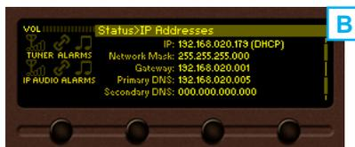
This operation will visualize the screen (B) containing information about the IP Address of the device.
